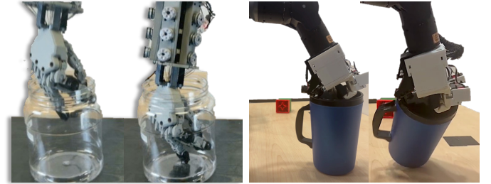
Fig. 12: Narrow Space Accessibility. CRAFT demonstrates the ability to fit into a narrow jar, while the bulkier Leap Hand V2 fails to enter the same workspace due to its rigid linkage size. Results reproduced with the help of the authors of Leap Hand V2 [25].
