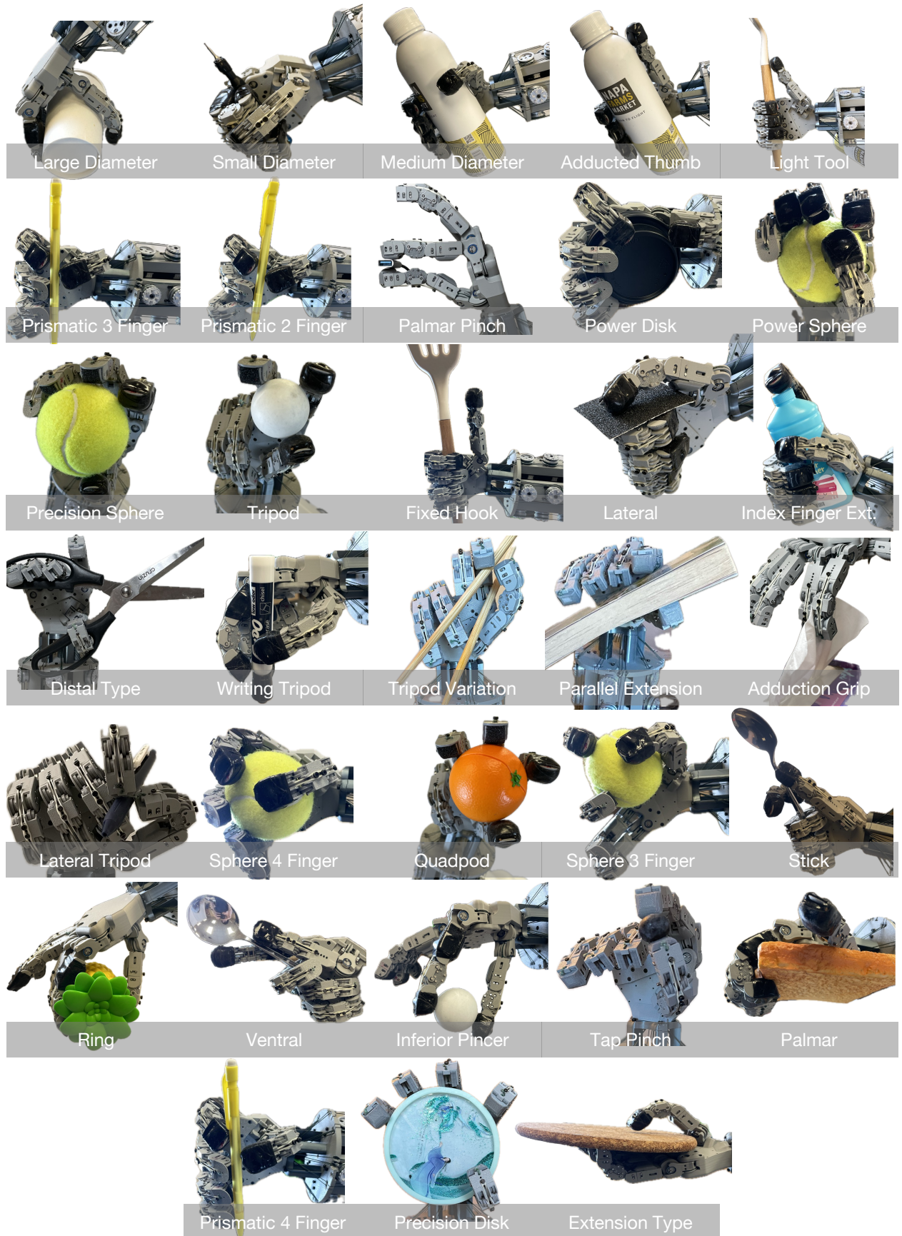
Fig. 9: Grasp Taxonomy Validation. CRAFT demonstrating 33 distinct grasp types from the Feix taxonomy [8]. The hand successfully executes a wide range of configurations, including power grasps (e.g., Large Diameter), precision grasps (e.g., Prismatic Pinch), and intermediate poses, confirming that the compliant design maintains the kinematic versatility required for general-purpose manipulation.
