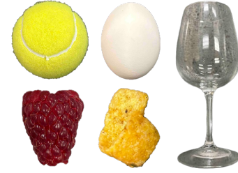
Fig. 7: Teleoperation User Study Objects. To validate real-world utility, we evaluate teleoperation performance on five objects: (1) a ball (rigid grasping), (2) a wine glass (large and fragile), (3) an egg (low friction and fragile), (4) a raspberry (small and deformable), and (5) a frito chip (extremely delicate).
